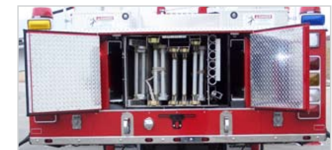
Low-Low Configuration with lap doors
