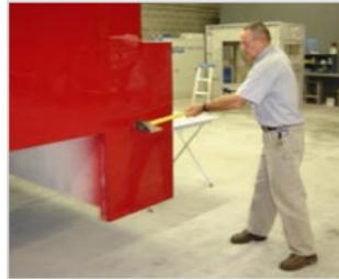
The body, constructed of Polyprene, is available in an extensive array of designs. The body and tank integrate into a unibody design, which eliminates the need and space required for supporting members, increases the space available for storage or water tank and lowers both the vertical center of gravity and hosebed height.
