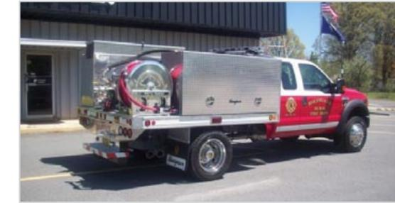
When you have a lot of rugged territory to protect, consider the Optimum® Brush Truck. It can rush to the off-road scene using four-wheel drive and a flat bed style set-up that includes water tank, pump, storage, reel(s), and ground sweeps.
