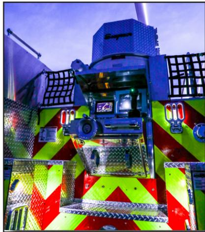
Rear Step Area Provides Easy Access to the Hosebed and Water Tower Secondary Controls.
